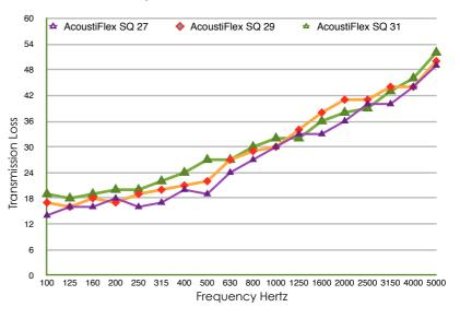
Note: The transmission loss at the frequencies of 100 and 125 Hertz have been estimated as site conditions were not suitable for measurement at these frequencies
